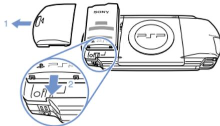
Align the tabs, and then slide the cover in the direction of the arrow until it locks firmly into place.
