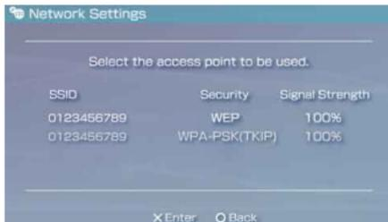
An SSID is a code or a name that is assigned to the access point. If you do not know which SSID to use or if the SSID is not displayed, contact the person who set up or maintains the access point.
