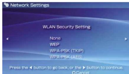
Security settings vary depending on the access point in use. To determine which settings to use, contact the person who set up or maintains the access point.
